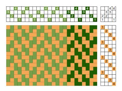
traditional broken twill (1, 2, 4, 3) and then switching another pair in the next four threads (1, 4, 2, 3). The drawdown on the left highlights the first eight-thread repeat in the darker green.
